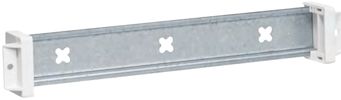
UT22C: 7,5mm DIN rail, insulated, insertable (212 mm length) 1-panel, adjustable depth up to 21 mm
