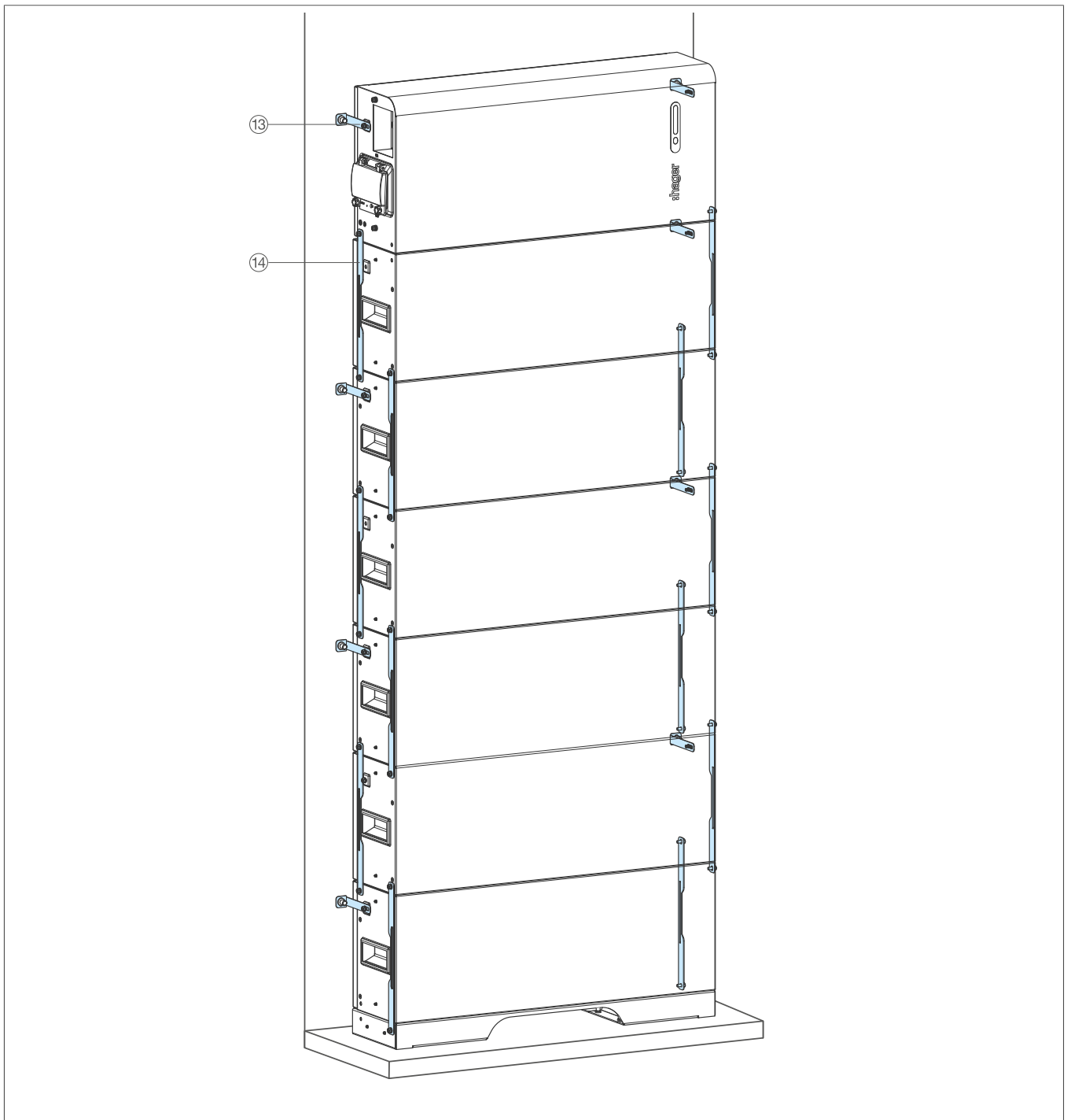
Fig. 22: Overview of all fasteners (see image)
