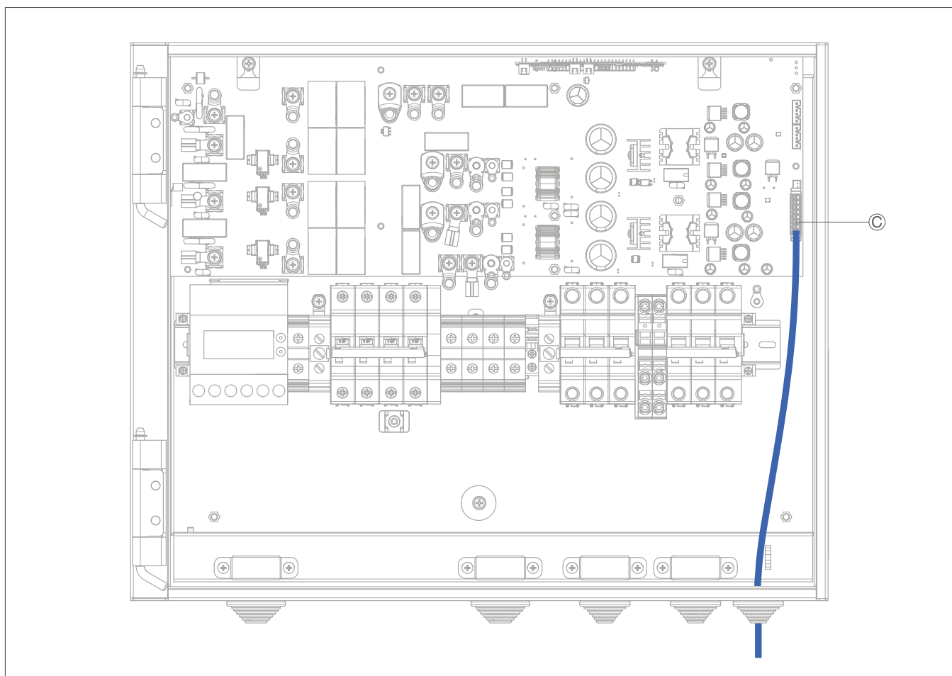
Fig. 31: ATS box, communication connection
